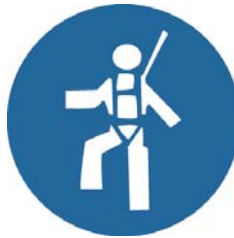
Compulsory personal protection against falls
