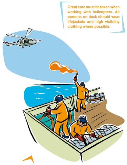
**USE A HAND FLARE** to indicate your position and wind direction to the helicopter, but only if requested. Never use a parachute flare.
